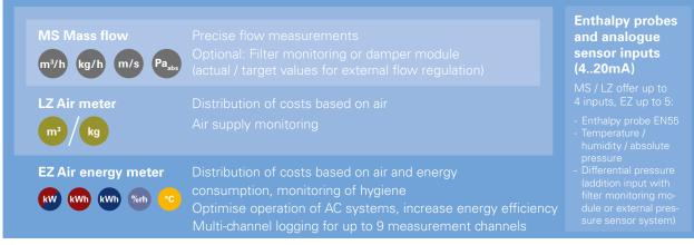
The Luftmeister range has to be functional in a wide variety of scenarios, therefore Luftmeister<sup>®</sup> developed three different models of the **Luftmeister<sup>®</sup> 55 and 57 series**. These are described in the table below. The **MS** model offers high precision mass (and volume flow) measurements. The **LZ** model adds an air meter function (air consumption in m<sup>3</sup> or kg). The **EZ** model (air energy meter) also calculates air energy contributions, see also page 6.
