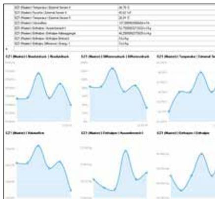
The professional PC software "Luftmeister Tool" can be used for commissioning as well as servicing and operation. This parameterises all inputs and outputs, reads out logger values to Excel in the CSV exchange format and displays the error, meter, and adjustment logbooks.
