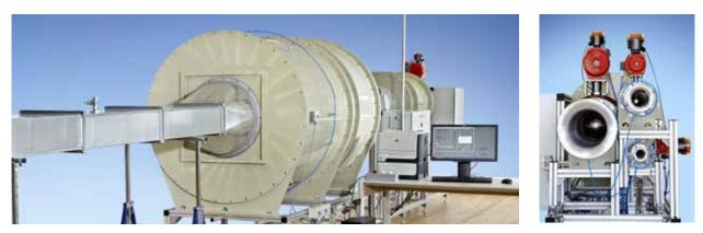
Every instrument in the Luftmeister® 55 series (MS55/LZ55/EZ55) is calibrated on a certified mass flow calibration stand.
